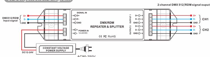
Note: When using RDM master to control several DMX slave devices, according to DMX512 protocol, a small metal film resistor of 90~120 Ω/1/4W should be welded at the end of each DMX signal line (between signal + and signal-).
